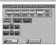
INSERT allows you to insert space and shift data that lie behind the FROM position further towards the end of the track (this is the exact opposite of DELETE). The empty measures you create can be "filled" using the COPY function or by recording new phrases in that area.
